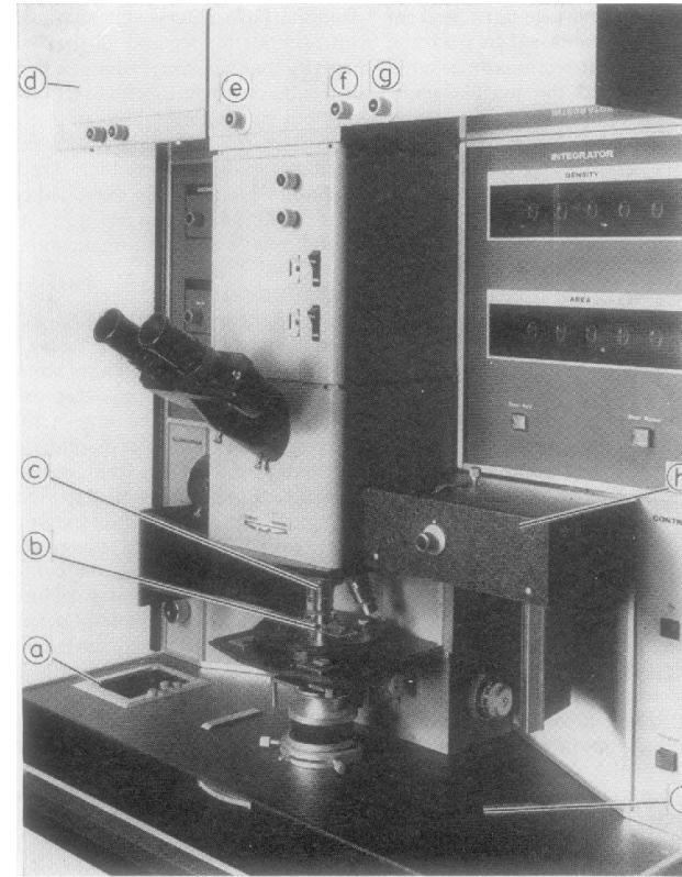
Fig. 1. Wako 140S scanning and interactive microdensitometer. (a)
